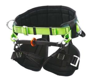
The TH 020 supported work belt for arborists, fitted with ergonomically profiled padding, adjusting buckles, side attachment buckles and anchoring point for suspended work. It uses aluminum adjustment buckles. Nor risk of accidental release. The TH 020 belt constitutes basic equipment for works at height, mainly on trees, poles, building structures, etc.
