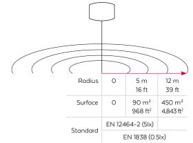
How to read the drawing: in a range of 12 m - 39 ft, being a surface of 450 m² - 4,843 ft², we guarantee a lighting in accordance with the EN 1838 standard.
